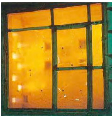
Glazed steel door and screen under fire test
